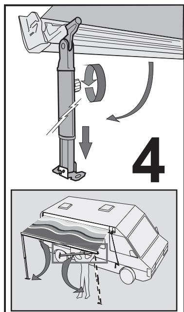
**EN** **Attention Security** The foot for leg A has been created to prevent its correct placing inside the housing of the lead bar during the closing phase of the awning. With an incorrect placing of the foot the lead bar wouldn't close completely; so we advised you to put it always into the housing properly with the base turned to the lead bar.
