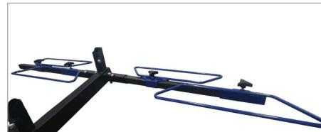
7. Once these components are assembled, you can confirm the position of the chassis brace on the chassis. Tighten 8x M8 nyloc nuts on the U-Bolts securing the bike rack assembly to the chassis.
