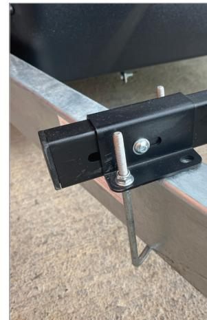
8. Tighten the 4x M8 nyloc nuts located on the bolts going through the slotted holes on the chassis brace, securing the lateral movement of the chassis brace on the upper chassis mounting brackets.
