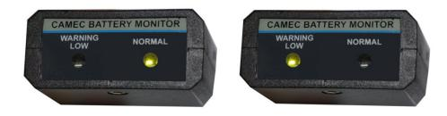
If the internal battery in the Break Away System is **not fully energised** a green light will illuminate and flash under the heading **Warning Low**. This light will continue to flash whilst your foot is applied to the brake and an audible alarm will sound if the brake is still held applied approx 10 seconds later and will beep for 5 seconds. Whilst the brake is continuously applied the audible alarm will beep for 5 seconds every 20 to 30 seconds.
