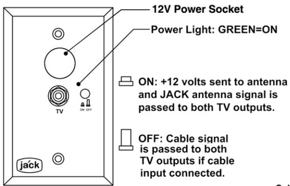
ON: +12 volts sent to antenna and JACK antenna signal is passed to both TV outputs.
