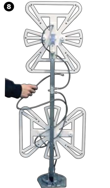
Continue to thread the coax in an S-curve. Thread the coax over and then under the boom.
