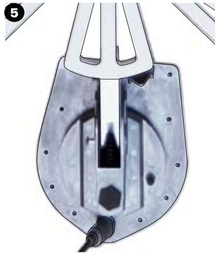
Insert the pin through the leveling bracket and the elevating gear. Push the e-clip over the end of the pin.
