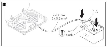
2. Add a 1 A fuse in the plus line near the battery.
