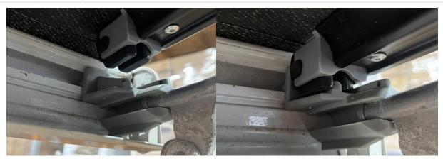
**Note:** The bracket goes over the inside plastic ridge. See in the image there are two ridges. If the bracket is on the outside ridge the AFK will not grip the fabric effectively.
