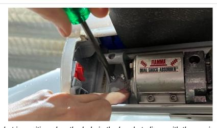
**Note:** The bracket is positioned so the hole in the bracket aligns with the awning fabric. This will ensure the AFK can grip firmly to the awning fabric when installed.
