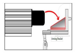
Open the 6 handles to allow the awning vinyl to be clamped inside the AFK.
