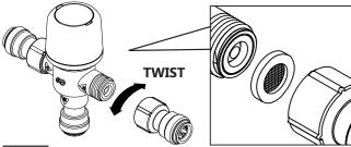
On the basis that the Tempering Valve is not moved from the system, the hot, cold and mixed pipe can be removed.
